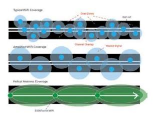
Tunnel WiFi uses circular polarization.
